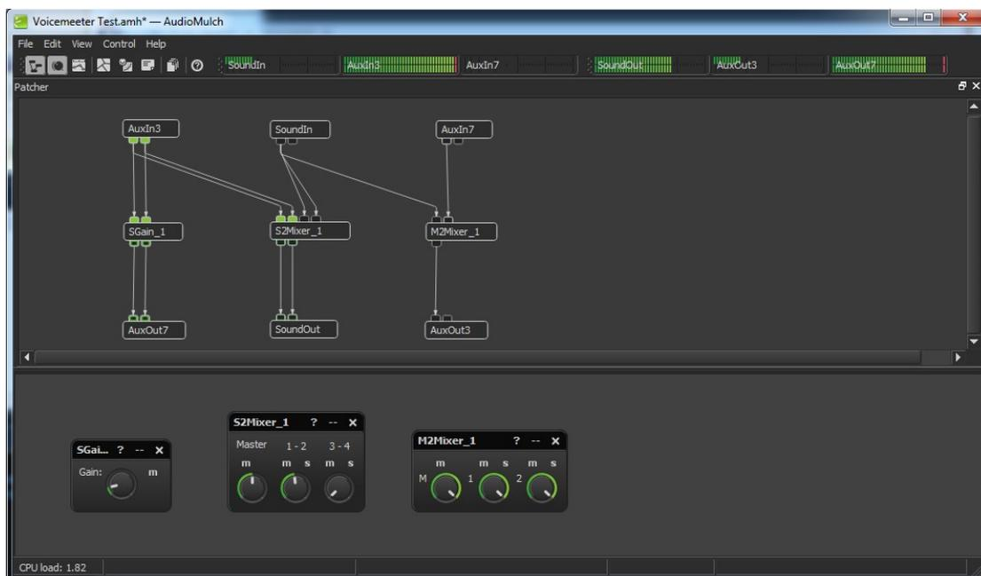
Figure 13—Audiomulch Patch Configuration.
